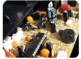
Control System – Auto Start/Stop, Auto Reverse when Paper Jam, Overload & Overheat Sensor
